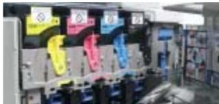
simple cartridges, which can be replaced without assistance
